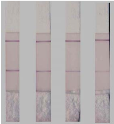
Figure 10. Dilution series of gold conjugate lateral flow devices. From left to right dilutions 1:10, 1:20, 1:40 and 1:80. Samples were of type A5 Allier (6/11/90) and detected with \alpha FMDV 1F10.
