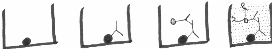
Figure 2. In ELISA concentration is measured via dual detection molecules (Y-shaped) binding to immobilized protein (big black dot). One of the detection molecules is linked to an enzyme (white dot) that catalyzes ( S \rightarrow P ) a detectable coloring of the surrounding liquid (small black spots).
