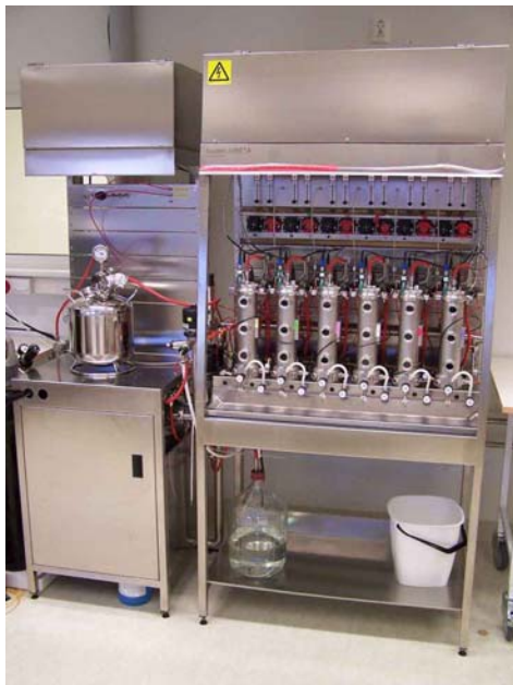
Figure 3: GRETA multifermentor with CIP-unit and growth medium vessel (Belach Bioteknik AB).
