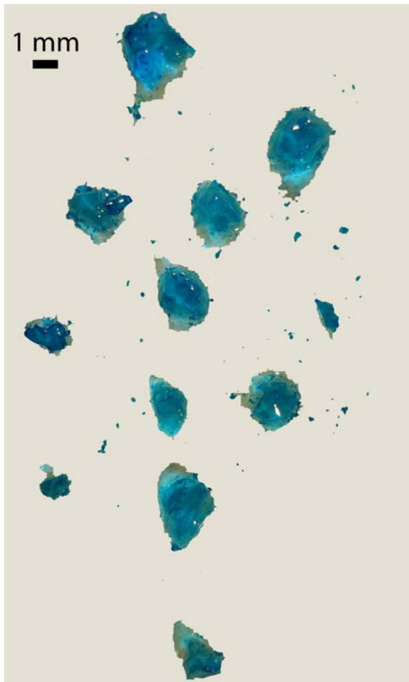
Figure 6: Image of Alcian Blue stained GelB particles. The image is photographed without any magnification.
