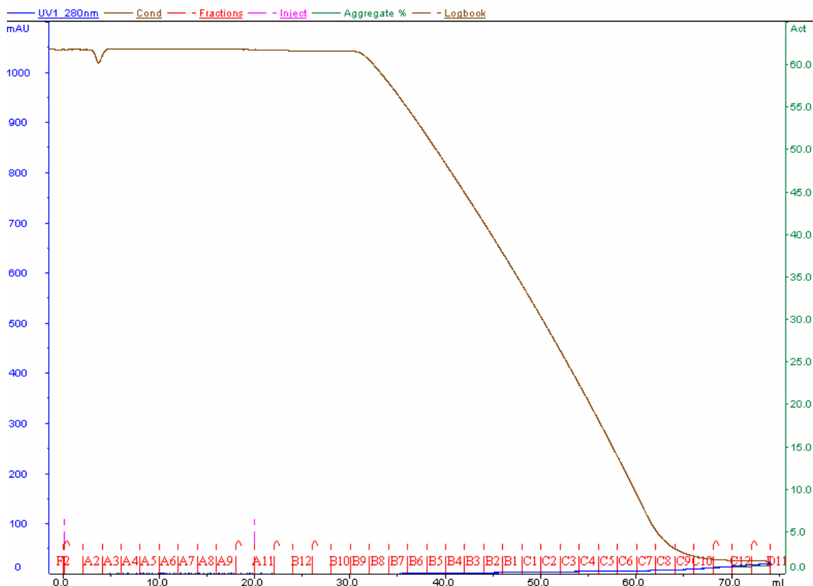
Figure 21. The chromatogram for B1 – Phenyl (31 µmol/ml) with 0.8 M ammonium sulphate, 50 mM sodium phosphate as binding buffer as binding buffer and 50 mM sodium phosphate without ammonium sulphate as elution buffer. Left axis and blue colour curve represents the absorbance at 280 nm in mAU, right axis and green colour curve represents the aggregate content in % and brown colour represents the conductivity. The protein did not elute in significant amounts.
