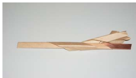
Figure 3. Rectangular copper wire wrapped with paper. With permission from Lena Melzer ABB Transformers Diagnostic Group.
