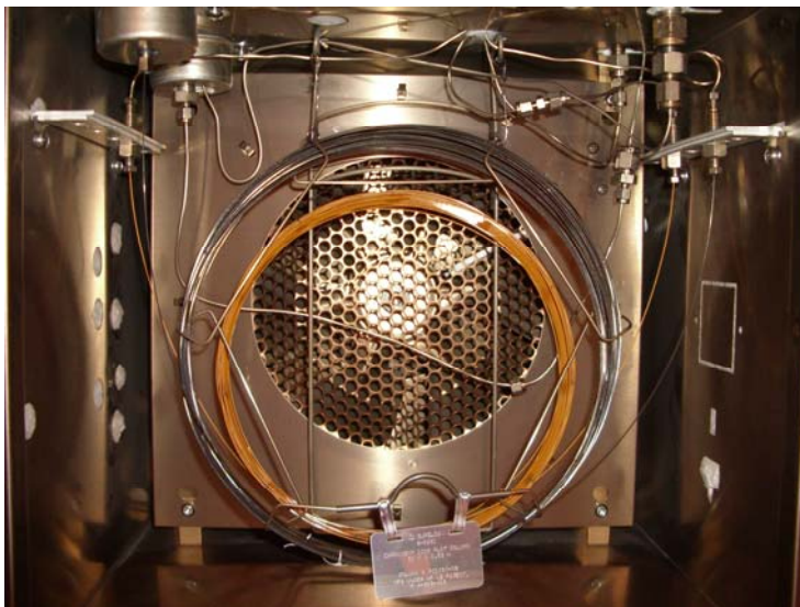
Figure 8. GC-oven interior for the regular DGA-setup. Picture used with permission from Lena Melzer ABB Transformers Diagnostic Group.
