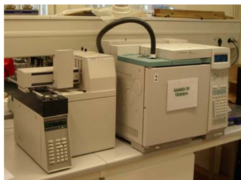
Figure 7. Headspace sampler connected to a GC via the transfer line. Figure used with permission from Lena Melzer ABB Transformers Diagnostic Group.
