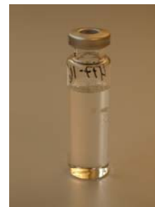
Figure 5. Headspace vial with mineral oil. With permission from Lena Melzer ABB Transformers Diagnostic Group.
