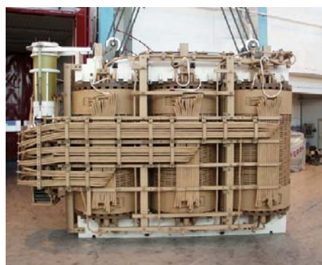
Figure 4. Paper insulated transformer without tank. Figure used with permission from Anna Nordh, security manager ABB Transformers.
