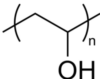
**Figure 2** The structure of polyvinyl alcohol
